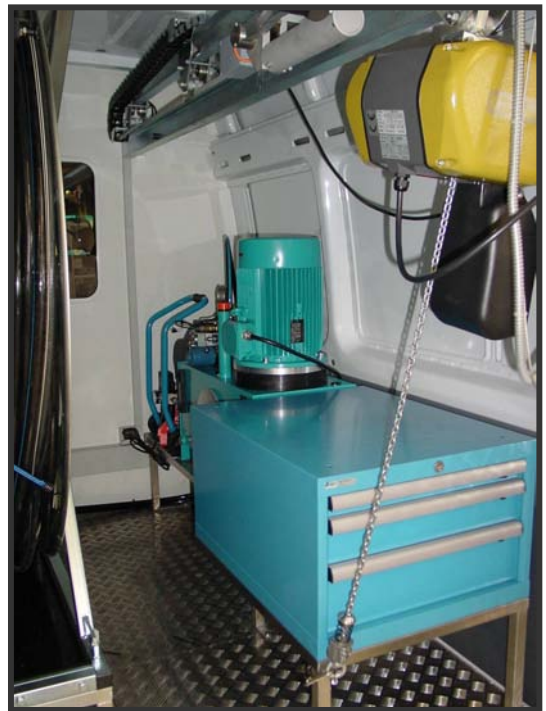
Aggregates: Cable drum, Hydraulic System, Water System, Crane, Tool Cabinet
